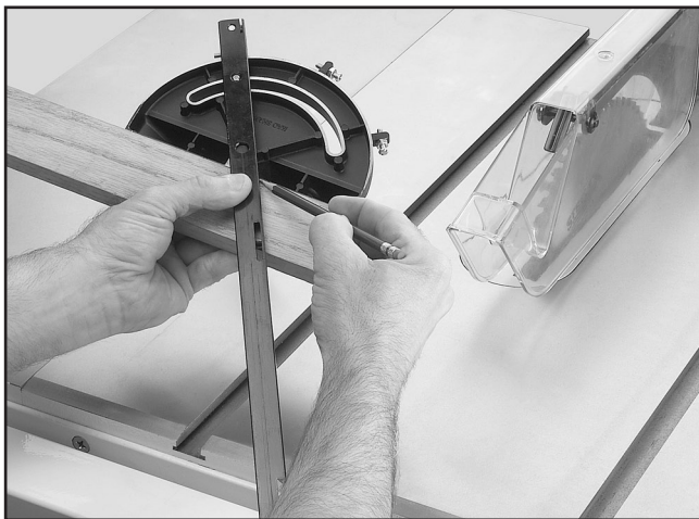
Figure 45. Example of marking miter line.
